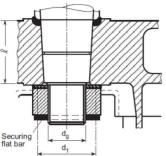
Fig 4.1.7 Cone coupling without key
