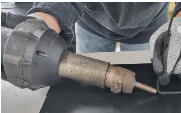
Figure 3-1 Hot gas welding using a torch separated from the electrode
