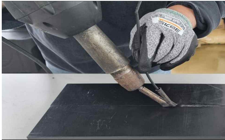
Figure 3-2 High-temperature gas string bead welding
