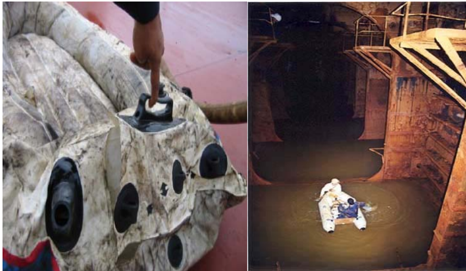
A damaged raft may result in capsize
