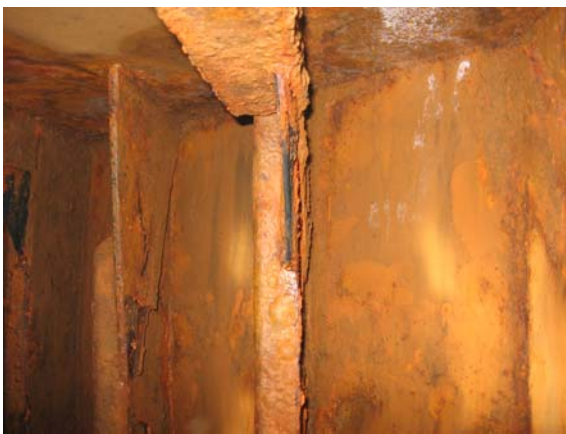
A typical stiffener & end bracket in a W.B.T. after chipping – cleaning may reveal the true thickness reduction it is subjected to
