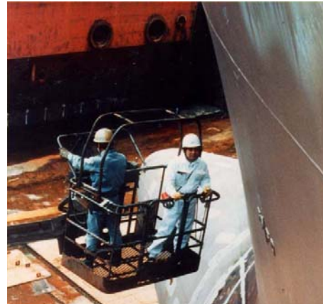
Typical Cherry Picker configuration and a surveyor performing close up survey on side shell plating
