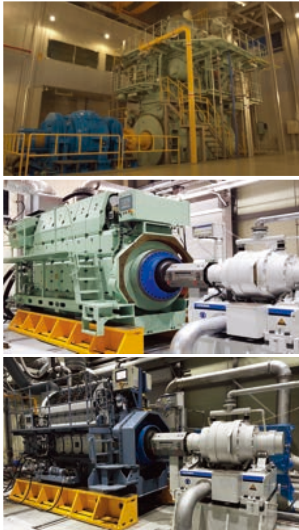
[Figure 7-1] Engine test benches within the center; top) slow speed diesel engine, middle) medium speed diesel engine, bottom) medium speed dual fuel engine
