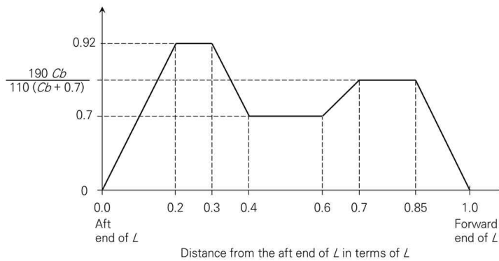
Figure 3 : Distribution factor of negative vertical shear force f_{q-neg}
