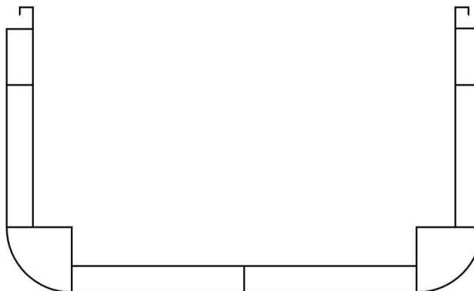
Figure 1 : Container ship of double side skin construction
