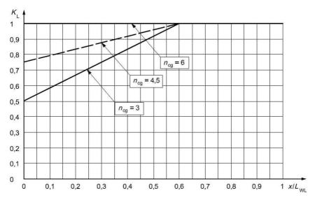
Fig 4.2 Longitudinal pressure distribution factor  $k_L$
