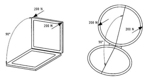
Fig 6.9 Hatch and hinge strength test
