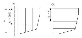
Fig 4.3 Watertight bulkheads
