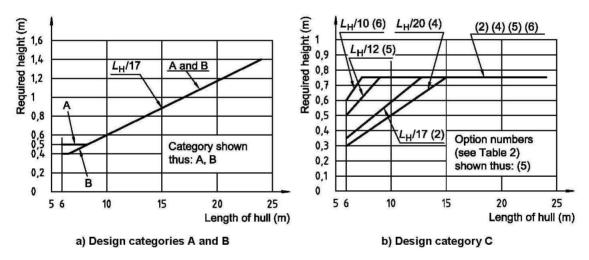
Fig 5.2 Required downflooding height - Design categories A, Band C
