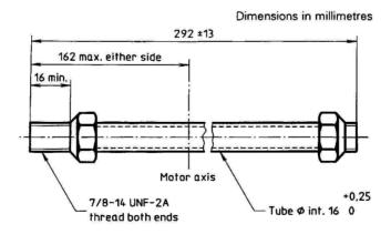
NOTE — The tube may be threaded equal length on both ends or reversible for port steering installation.
