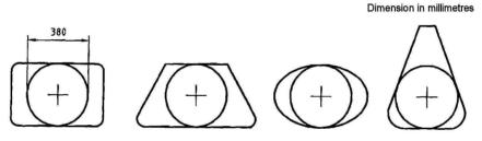
Fig 11.2 Measurement of minimum clear opening
