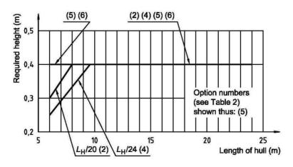
Fig 5.3 Required downflooding height - Design category D
