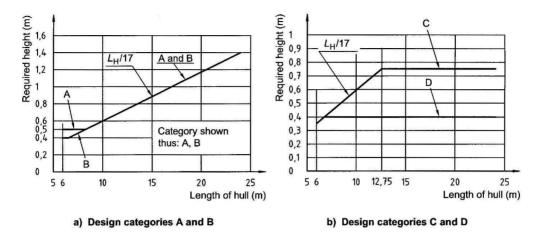
Fig 5.6 Required downflooding height
