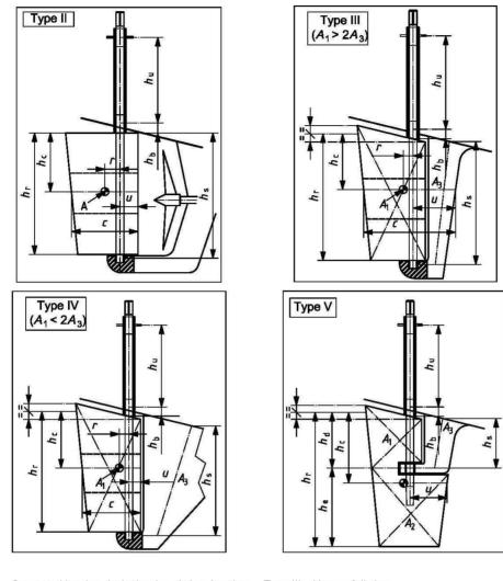
Type II Supported by skeg (solepiece) and skeg bearing Type III Narrow full skeg Type IV Wide full skeg Type V Partial skeg
