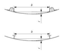
Fig 4.5 Measurement of convex curvature
