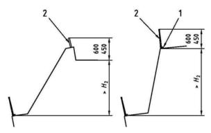
c) Actual height  $> H_2$ : foot-stop and guard-rail/line required
