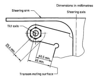
Fig 7.2 non-sailing-mounted steering tilt axis
