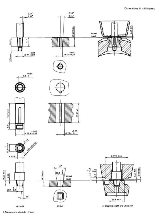
Fig 7.3 Steering shafts and steering-wheel hubs
