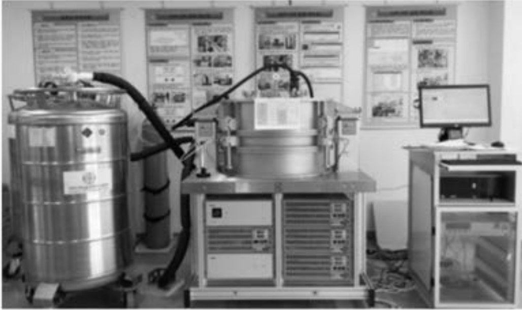
Figure 6.11 Commercial guarded hot plate method apparatus (C177)
