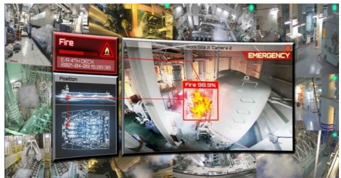
AI-based Video Fire Detection System <Source : HD KSOE>
