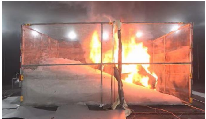
Test for fixed high-expansion foam system <Source : IMO SSE 9/INF.4>
