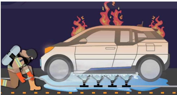
Underbody Water Spray Equipment <Source : Guide for Responding to EV Fires, National Fire Research Institute, 2023>
