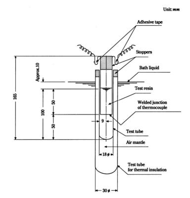
Fig 1.1 Testing Apparatus for Hardening Characteristics at Room Temperature
