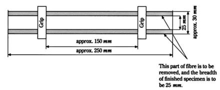
Fig 1.5 Tensile Test Sample of Roving Cloth
