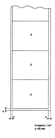
Fig 1.2 Selection of Test Specimens from Fibreglass Reinforcements
