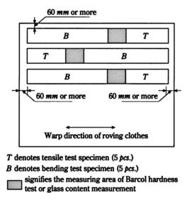
Fig 2.1 Location of Selection of Test Specimens
