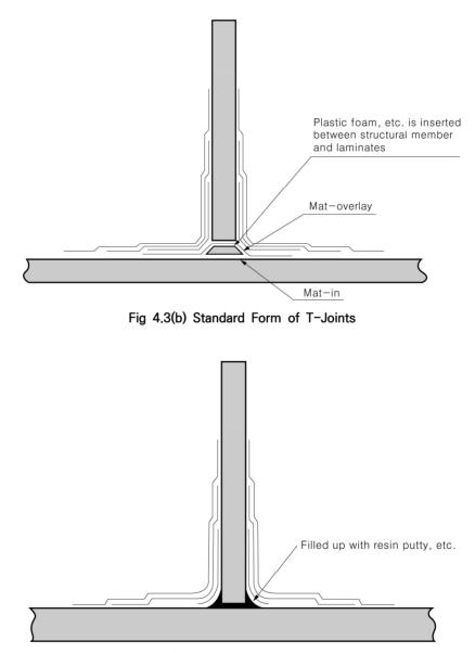
Fig 4.3(c) Standard Form of T-Joints
