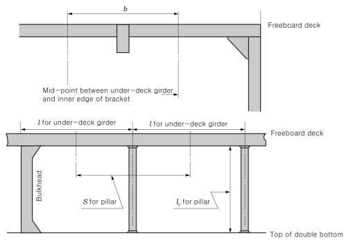
Fig 11.1 Measurement of b, l, S, and  $l_0$
