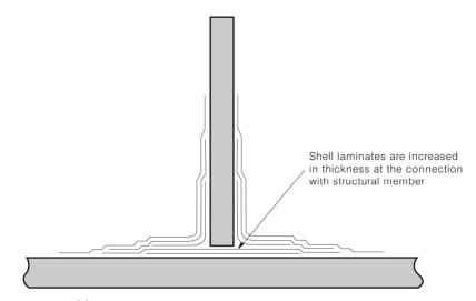
Fig 4.3(a) In Case Consideration is to be paid to Load or Vibration
