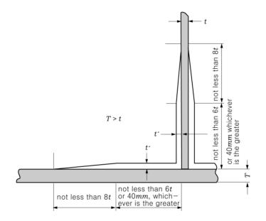
Fig 4.1 Dimensions of Overlap of T-Joints
