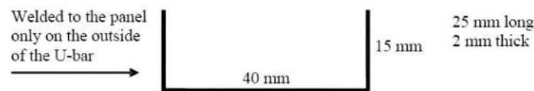
Fig 3.30.1 Welding of U-bar
