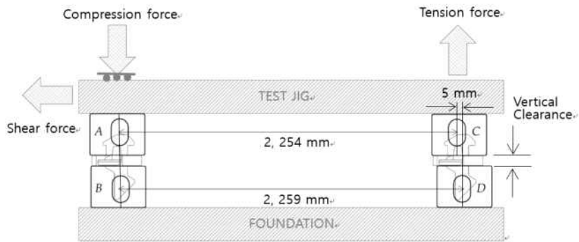
Fig. 3.25.1 Configuration of test equipments (2019)
